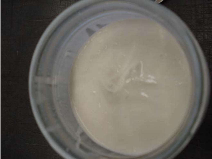
Thawed Water-Based Adhesive Showing Solid Consistency
