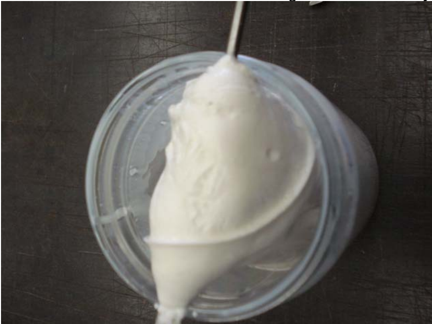
Thawed Water-Based Adhesive Showing Solid Consistency
